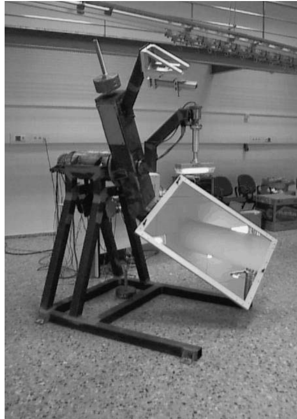
Fig 6. Automated goniophotometer (auxiliary mirror not shown).
