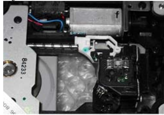
Figure 1. The two-actuator optical disk drive
