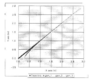
Fig. 5. Change of tracking response according to the change of gain
