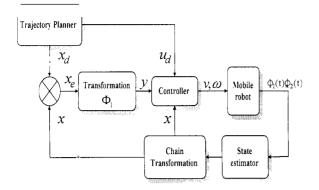
Fig 2 Block diagram of trajectory controller
