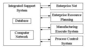
Fig. 3. the structure of IAS in Handan Iron & Steel Corporation
