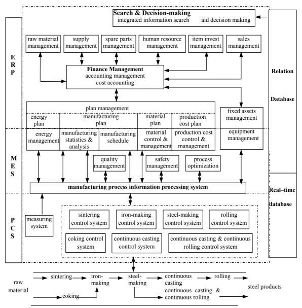
Fig.4 the function figure of IAS in Handan Iron & Steel Corporation
