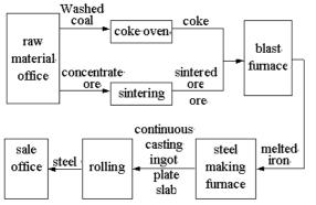
Fig. 2. Technological flow diagram in Handan Iron & Steel Corporation
