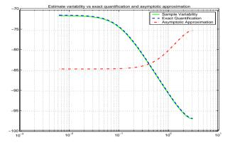
Fig. 1. Variability of Fixed Denominator Estimate - First Order Example. True variability vs. theoretically derived approximations. Solid line is Monte–Carlo estimate of true variability, dashed line is quantification (26), dash-dot line is asymptotic-based approximation (12).
