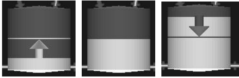
Figure 4: Visualization of the actual and desired fill-up level (L) (left: actual L lower than desired L; center: actual L = desired L; right: actual L higher than desired L)
