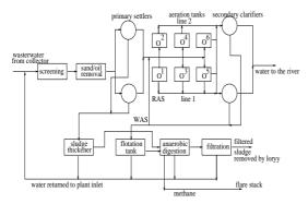
Figure 3. Schematic diagram of the wastewater treatment plant
