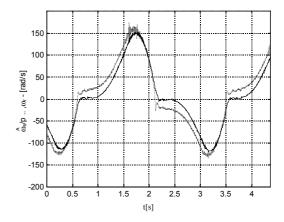
Fig. 7. Step load - estimated value of stator frequency and actual value of speed.
