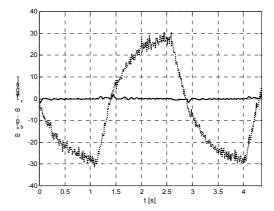
Fig. 5. Locked rotor - estimated value of stator frequency and actual value of speed
