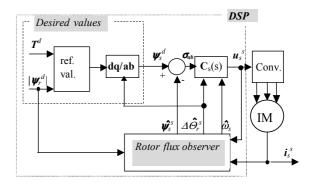
Fig.1. Proposed control scheme with the included closed-loop observer
