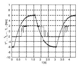
Fig. 6. Step load - desired and estimated value of IM torque  $T_e$  and load torque  $T_L$ .
