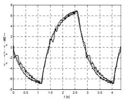
Fig. 4. Locked rotor - desired, estimated, and actual value of IM torque  $T_e$ .
