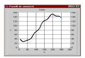
Fig.4. Simulated and real trajectories of the robot
