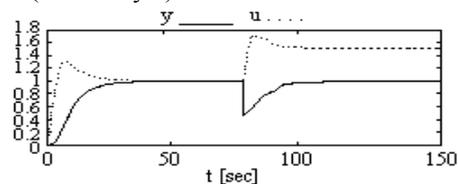
Fig. 10.  $y$  and  $u$  versus time for CS with M-PI-FC (case study 2).
