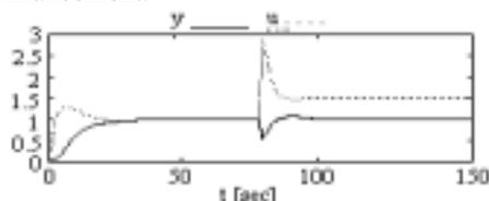
Fig. 9.  $y$  and  $u$  versus time for CS with PI controller (case study 2).
