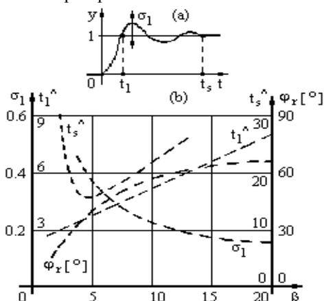
Fig. 2. Definition of control system performance indices (a) and their variations versus  $\beta$ .
