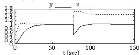
Fig. 11.  $y$  and  $u$  versus time for CS with TS-PI-FC (case study 2).
