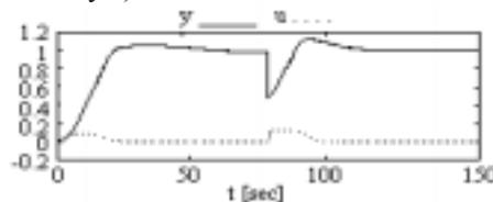
Fig. 8.  $y$  and  $u$  versus time for CS with TS-PI-FC (case study 1).
