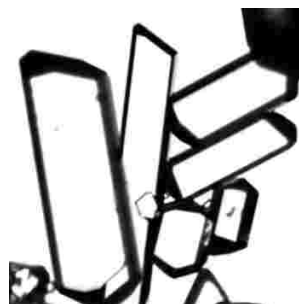
Fig. 1. Photograph of paracetamol crystals taken from a batch crystallizer (paracetamol is the active ingredient in Tylenol).
