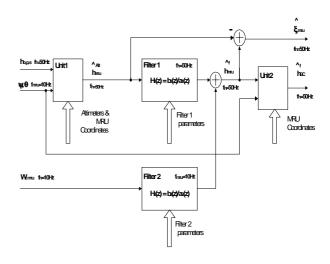
Fig.2. Algorithm structure for filtration of measurements of altimeters and vertical accelerometers.
