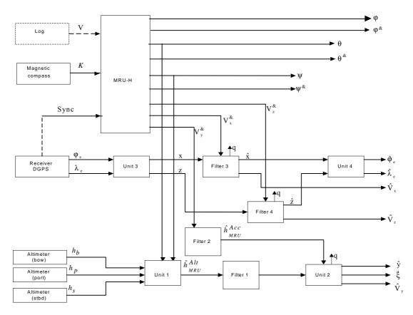
Fig.1. Block-diagram of integrated measurement system.
