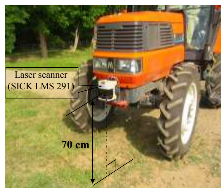
Fig.7. Two-dimensional laser scanner attached to the robot tractor
