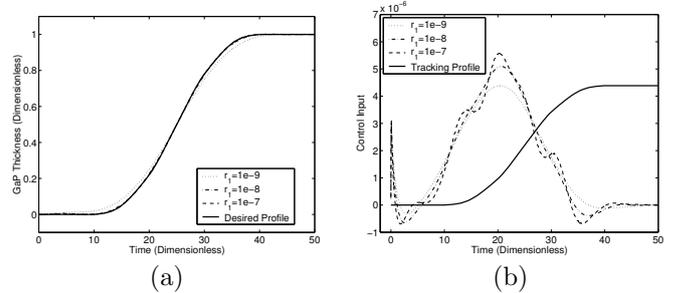
Fig. 4. Each dimensionless time unit corresponds to 0.1 s. (a) Controlled growth film thickness profiles for various  $r_1$  values. (b) Feedback control inputs for various  $r_1$  values plotted against not-to-scale film thickness tracking profile
