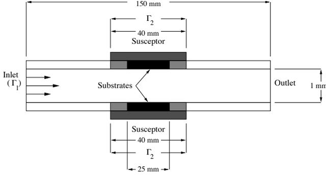
Fig. 3. HPCVD reactor side-view cross-section (not to scale). The width of the reactor is 50 mm.
