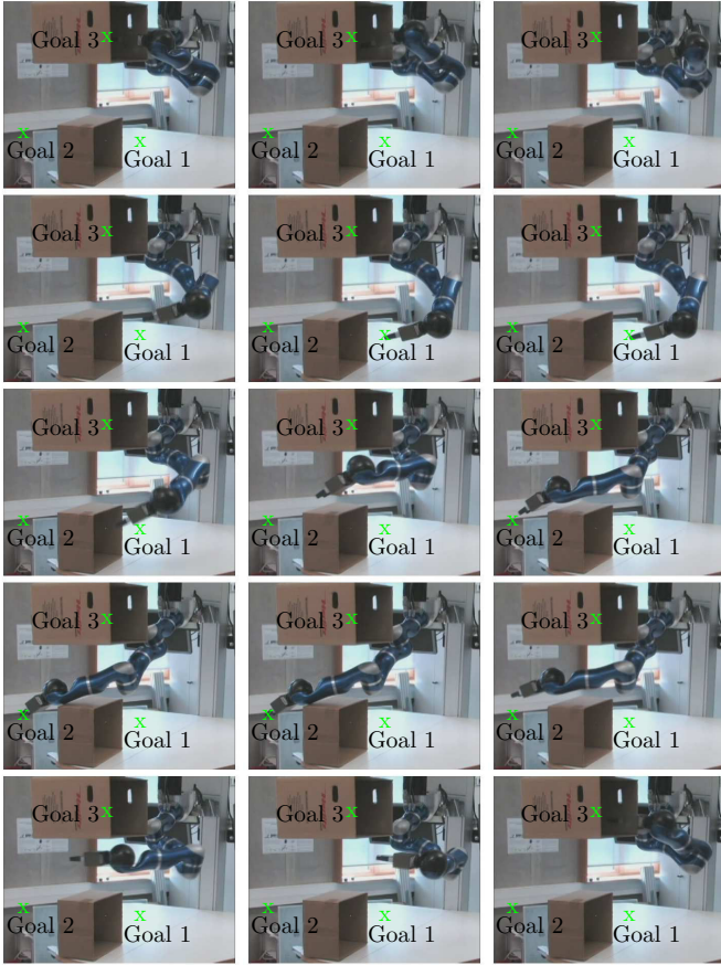
Fig. 12. The task is to reach all three goals in real-time. The robot is able to perform this task without getting stuck in a local minimum.
