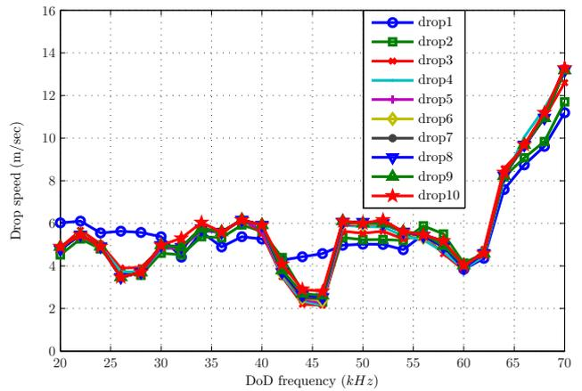
Fig. 11. Standard pulse: Jetting 10 drops at different DoD frequencies (20-70 kHz).
