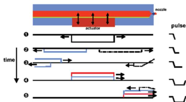
Fig. 2. Drop jetting mechanism
