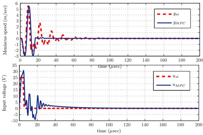
Fig. 7. System response for jetting one drop.
