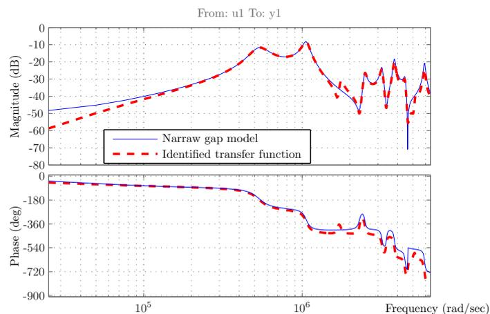
Fig. 5. Frequency response of the narrow gap model (solid line) and the fitted transfer function(dash line).
