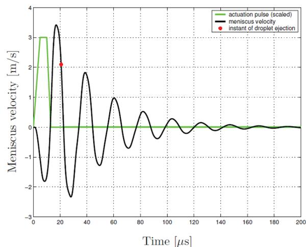
Fig. 3. System response for the standard pulse
