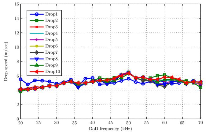
Fig. 12. Proposed pulse: Jetting 10 drops at different DoD frequencies (20-70 kHz).
