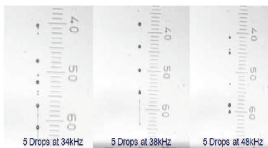
Fig. 4. Jetting 5 drops at different DoD frequencies.
