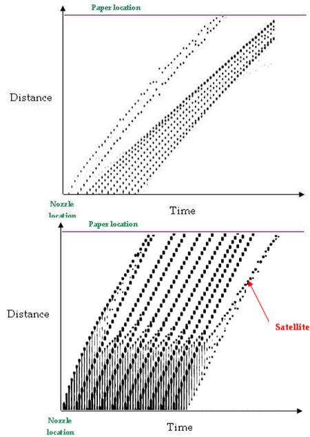
Fig. 10. Drop time history for jetting 10 drops at 42 kHz with standard pulse (Upper plot) and proposed pulse (bottom plot).
