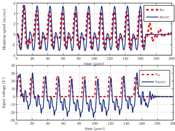
Fig. 8. System response for jetting 10 drops at 60 kHz.
