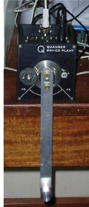
Fig. 1. A single link manipulator and a servo-motor.
