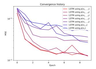
Fig. 6. LSTM convergence history as a function of number of pressure readings used to train the network.
