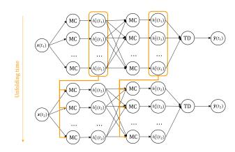
Fig. 1. An example of a two layer LSTM with each layer containing C memory cells (MCs), followed by a time-distributed (TD) layer. Temporal dependencies are highlighted in yellow.
