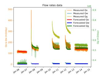
Fig. 11. Multiphase rates forecast for the LSTM trained on first 2 flow periods. Spurious oscillations are plotted semi-transparent.
