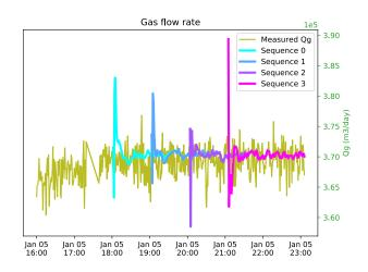
Fig. 12. First output sequences of zoomed LSTM gas rate forecasts.
