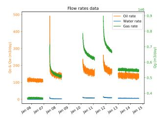
Fig. 10. Multiphase rates for the variable rate well test.
