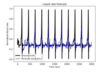
Fig. 5. Feedforward ANN liquid rate forecasts using a single pressure readings as input.
