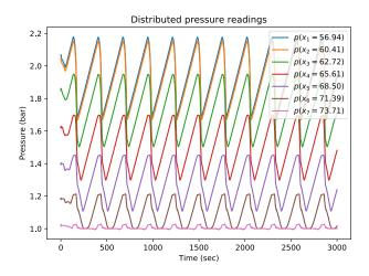
Fig. 3. Pressure data used as input to forecast the flow rates.
