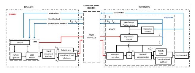
Fig. 3. Tele-operation system block diagram.
