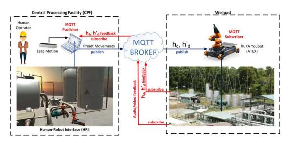
Fig. 2. Bilateral tele-operation system architecture.
