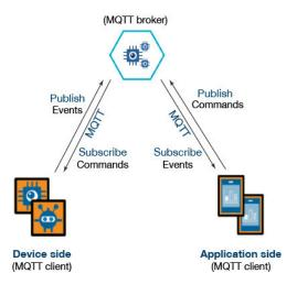
Fig. 1. MQTT Architecture
