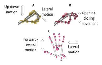
Fig. 5. Slave control movements. A) Up-down and lateral motion for the robotic arm. B) Opening-closing movement for the two-finger grip. C) Forward-reverse motion for the omnidirectional platform.
