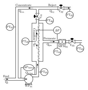
Fig. 1. Considered membrane filtration configuration.
