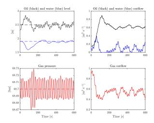
Fig. 5. Case 2 - state variables and manipulated variables for constant disturbance in the prediction horizon
