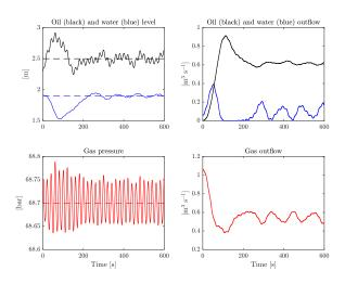
Fig. 6. Case 2 - state variables and manipulated variables for time-varying disturbance in the prediction horizon
