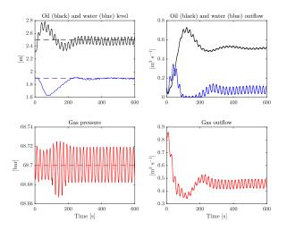
Fig. 3. Case 1 - state variables and manipulated variables for constant disturbance in the prediction horizon
