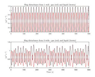
Fig. 2. Slugging inflows of liquid and gas to the separator
