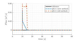
Fig. 5. Bottom-hole flow estimation error.
