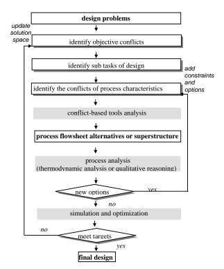
Figure 3. The paradigm of conflict-based method for chemical process synthesis
