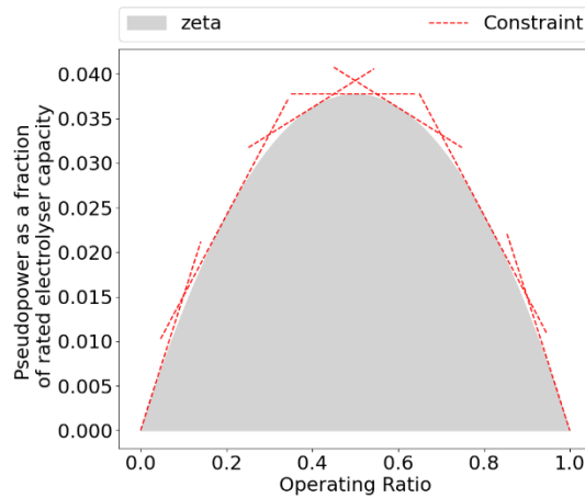
Figure 1 - Suitable region for the definition of the pseudopower. Acceptable values lie within the grey curve, and are constrained there by the linear constraints represented using dashed lines.
