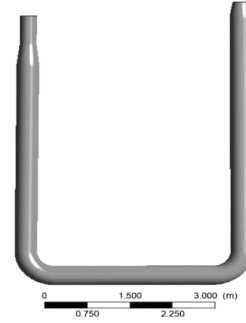
Figure 2: Fluid domain for the computational model
