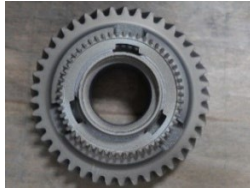
Figure 1: gear box pinion (23MnCrMo5 steel)
