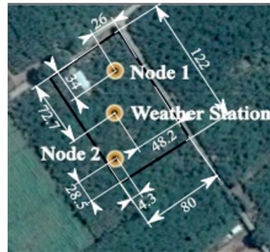
Figure 1: Nodes and weather station distribution, dimensions in meters.
