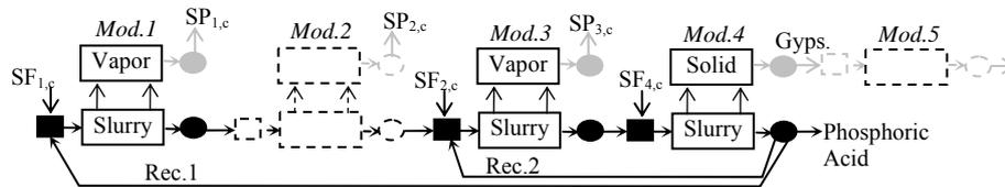
Figure 3: Existing industrial phosphoric acid production flowsheet and potential design options
