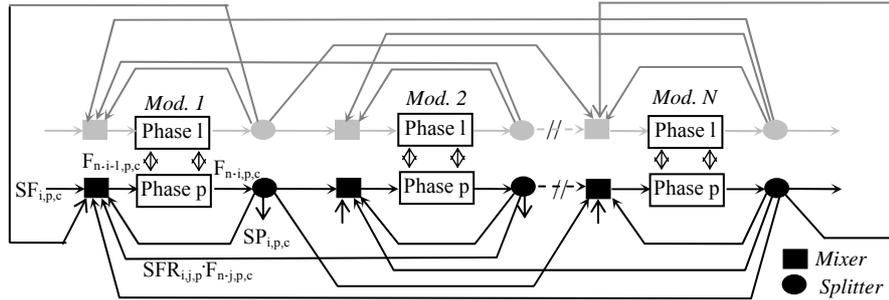
Figure 2: Process flowsheet of generic process modules and connectivity options
