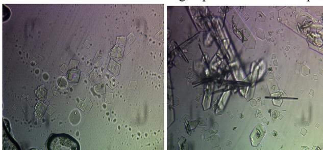
Fig. 2 Polymorph transition for L-glutamic acid captured in real-time, from  $\alpha$  form (left) to  $\beta$  form. The right figure shows mixed  $\alpha$  and  $\beta$  indicating transition being taking place.
