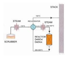
from about 200 to 300°C. The efficiency of destruction of nitrogen oxides and dioxides is high in the catalytic reactor, but the reactor also has a certain disadvantage in its sensitivity to catalytic poisons and in a necessity to include it in the technology line only at a point where the flue gases is free from particulates, which practically means behind mechanical and chemical cleaning operations (Fig.2).
