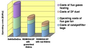
All running cost linked with a one year operation of the unit is included. The operating cost of the catalytic filtration DeNOx/DeDiox rises due to the reheating of flue gases to the required temperature of the reaction of about 250 °C and the cost linked with the increased pressure drop (Fig.5).
