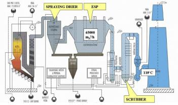
Fig.1 Configuration of an incinerator
