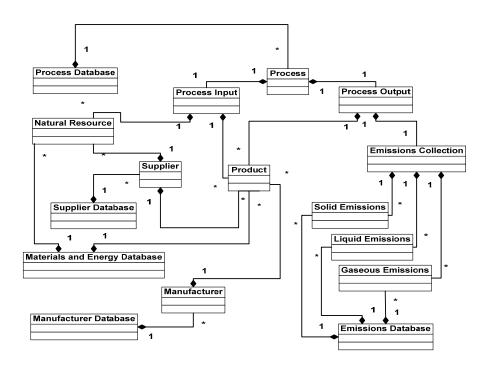
Figure 1. UML Entity-Relationship model of LCA Data Model
