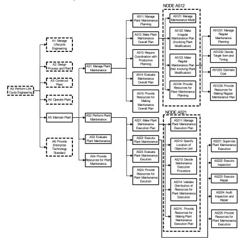
Figure 2 Structure of Activities for Plant Maintenance
