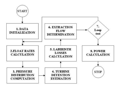
Figure 1. Cogeneration steam turbines calculus algorithm
