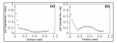
Fig. 4. 2-D plots for the variations of ferric (a) and zinc (b) concentration versus distance from the particle surface to the bulk of liquid
