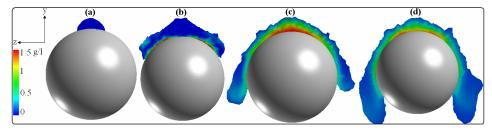
Fig. 2. Snapshots of the concentration profile of ferric ion. Realizations each separated by 0.01 s and the simulation was carried out for the inlet air velocity of 0.01 m/s.
