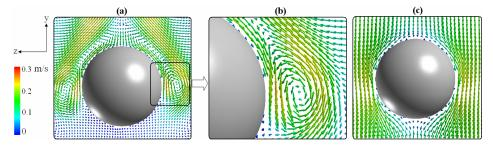
Fig. 5. Vector plot of liquid velocity field around single particle. Here the inlet air velocity is 0.5 and 0.01 m/s for parts a and c respectively. To obtain better visualization of flow field around the particle, the flow patterns marked in (a) is magnified and represented in (b).
