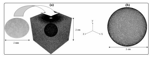
Fig. 1. (a) grid and dimensions of the computational domain and liquid entrance, (b) particle grid.
