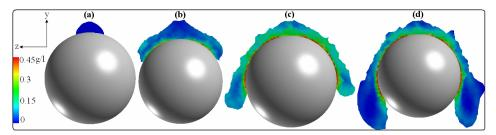
Fig. 3. Snapshots of the concentration profile of zinc ion on the surface of particle. Realizations each separated by 0.01 s and the simulation was carried out for the inlet air velocity of 0.01 m/s.
