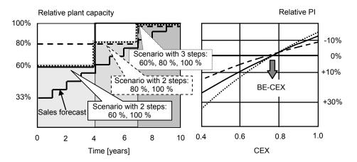
Figure 3: Typical plant expansion scenarios for a given linear and monotonically increasing sales forecast curve and corresponding relative *PI*.
