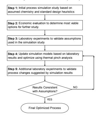
Figure 1. Flowchart for integrating process simulation work with experiments.
