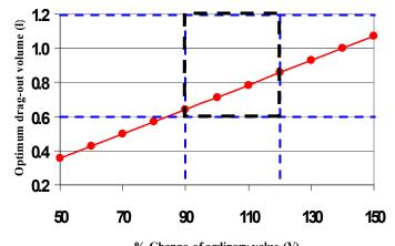
% Change of ordinary value (V) Figure 3 Optimal volume of drag-out with respect to water volume change
