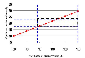
Figure 2 Optimal volume of rinse water with respect to drag-out volume change
