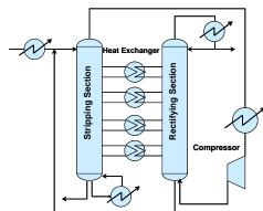
Fig.3 Schematic picture of a single HIDiC distillation column constituted by an internal heat integration method.
