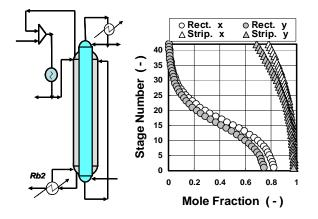
Fig.9 Stagewise variation of c-pentane concentration in the rectifying and stripping sections of the second HIDiC column:
