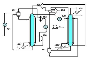
Pr: Preheater, Cd: Condenser, Fl: Flash Drum, Cm: Compressor, Rb: Reboiler, Sp: Splitter, Mx: Mixer
