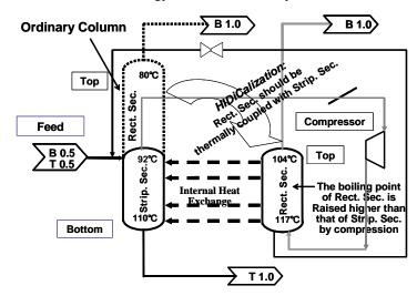
**Fig.1** Principle of internal heat integration by pumping the latent heat discharged from the rectifying section up to the stripping section. The numerals given as an example are the roughly-estimated compositions in mole fraction and boiling points of a binary mixture of benzene and toluene.
