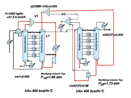
Fig.4 Schematic picture of a total HIDiC system devised in place of C5-splitter.
