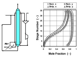
Fig.8 Stagewise variation of c-pentane concentration in the rectifying and stripping sections of the first HIDiC column:
