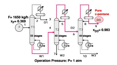
Fig.2 The existing C5-splitter for extracting pure c-pentane as the third overhead product D3 from a twelve-component mixture of petroleum hydrocarbons.
