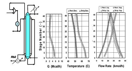
Fig.7 Stagewise variation of internal heat exchange rate, tray temperature and flow rates of vapor and internal reflux liquid in the second HIDiC rectifying and stripping sections
