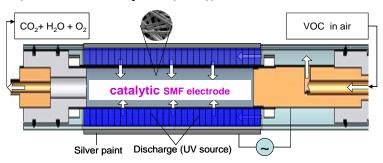
Fig.1. Schematic representation of the novel DBD reactor with catalytic SMF electrode
