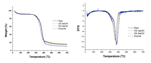
Figure 2- (a) Tg and (b) DTG curves for raw, NaOH and enzyme treated fibers.
