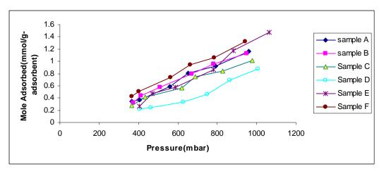
Figure 1: Experimental adsorption isotherm for CO<sub>2</sub> on six different adsorbents.
