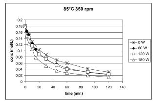
Figure 2. The concentration of ferric iron as a function of time for experiments performed with different ultrasonic power. Experiments were performed at 85°C with an agitation rate of 350 rpm.
