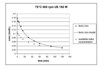
Figure 1. The measured concentration of ferric iron as a function of time (the filled symbols). The line represents the modelling result and the open symbols are the calculated values for sphalerite.
