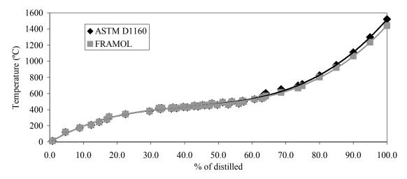
**Figure 4:** True Boiling Point Curves from ASTM and FRAMOL correlations and extensions to 100% of distillate for Beta 540°C+ petroleum.
