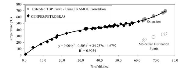
Figure 3: Extension of the true boiling point curve for Beta 540°C+ petroleum through molecular distillation considering FRAMOL correlation.
