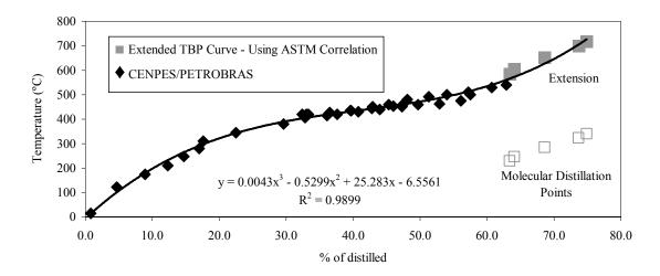
Figure 2: Extension of the true boiling point curve for petroleum Beta 540°C+ through molecular distillation considering ASTM D1160 correlation.
