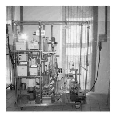
Figure 1: Molecular distillation apparatus (UIC-Gmbh KDL 5 unit)
