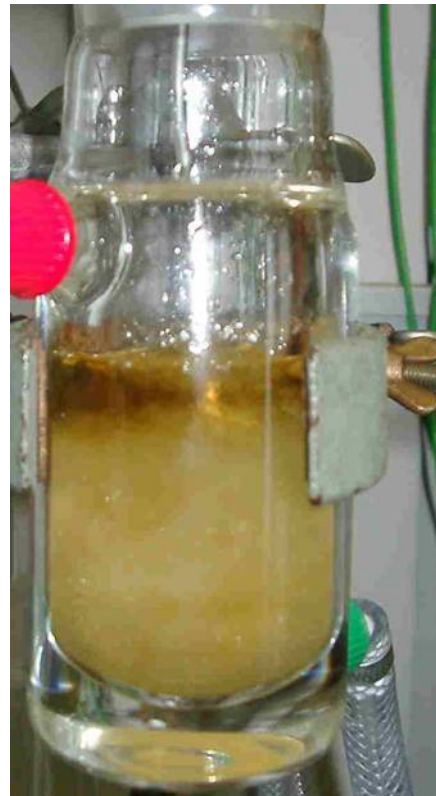
Figure 3: Static layer crystallization of EMIM-Cl, m_{\text{Feed}} = 50 g
