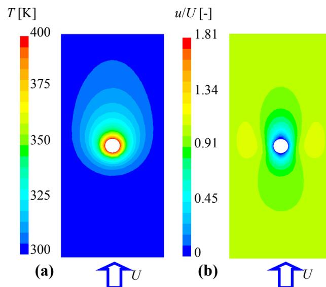
**Fig. 3** (a) Temperature and (b) velocity distributions ( $Re = 10$ , fine mesh)
