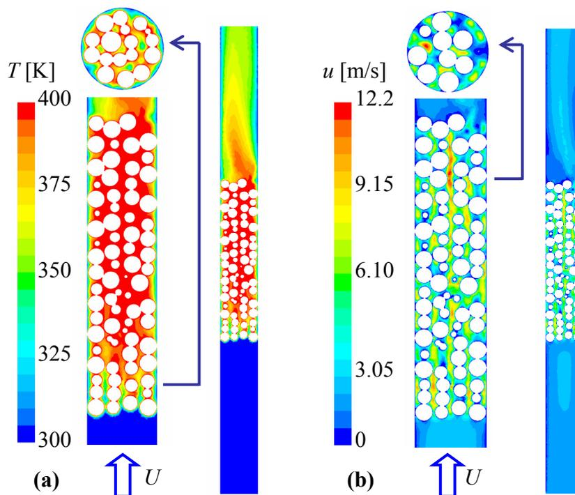
**Fig. 5** (a) Temperature and (b) velocity distributions ( $Re = 200$ , fine mesh)
