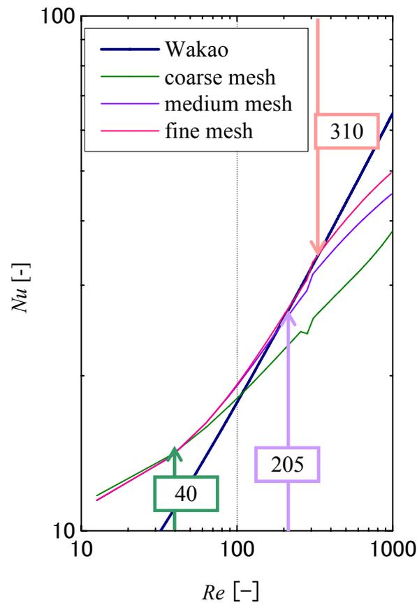
**Fig. 7**  $Re$  conditions for each mesh density to predict the accurate heat transfer.
