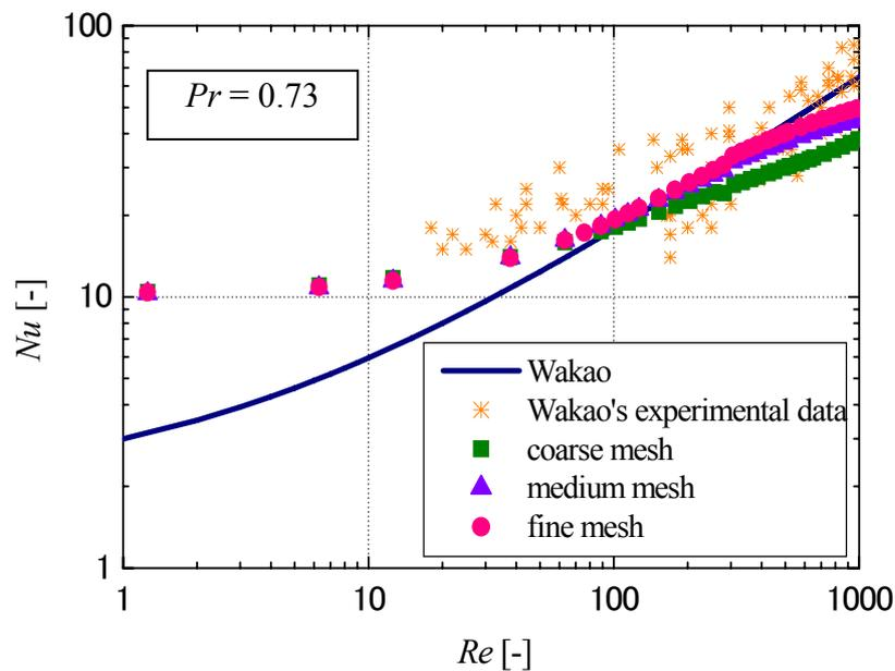
**Fig. 6** Comparison of CFD-predicted  $Nu$  with the correlation and experimental results
