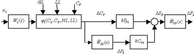
Fig.2. Block diagram of the linearized unit model
