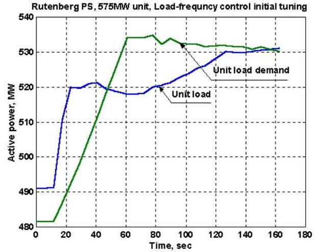
Fig.1. Unit 575MW responses with the tuned LFC. The unit load demand is equal to  $L_{SP} + \varepsilon_F$
