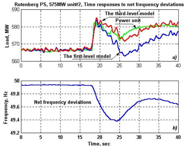
Fig.6. Plot of simulated and measured responses of 575MW unit No.2 to net frequency abrupt deviations
