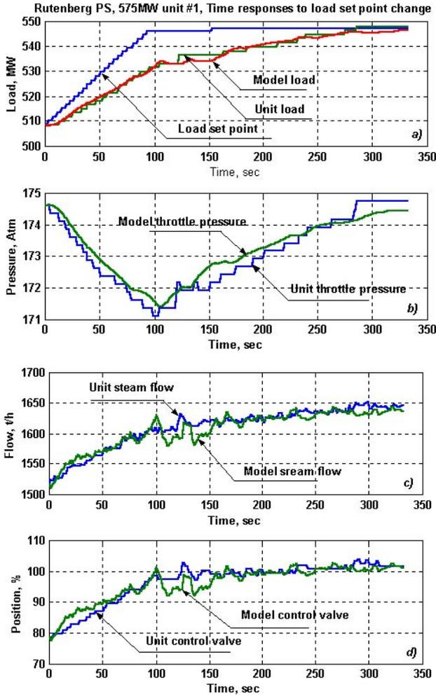
Fig.4. Plot of simulated and measured responses to the load set point  $\Delta L_{SP}$  (a);  $\Delta P_T(t)$ ; (b)  $\Delta S_F(t)$ ; (c)  $\Delta C_V(t)$
