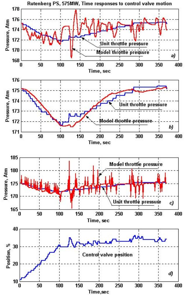
Fig.3. Plot of simulated and measured throttle pressure responses: a)  $\sigma = 1$  sec ; b)  $\sigma = 100$  sec ; c)  $\sigma = 120$  sec
