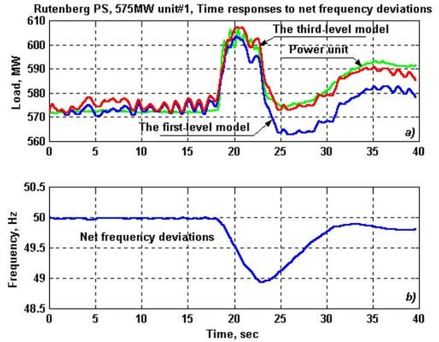
Fig.5. Plot of simulated and measured responses of 575MW unit No. 1 to net frequency abrupt deviations
