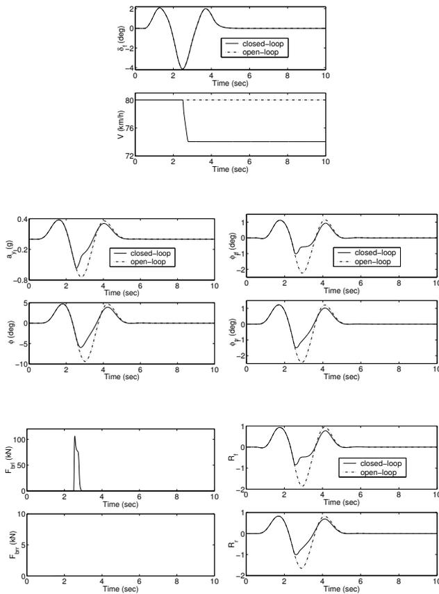
Figure 4: Time responses to double lane change steering input
