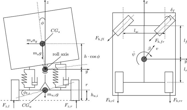
Figure 1: Rollover vehicle model
