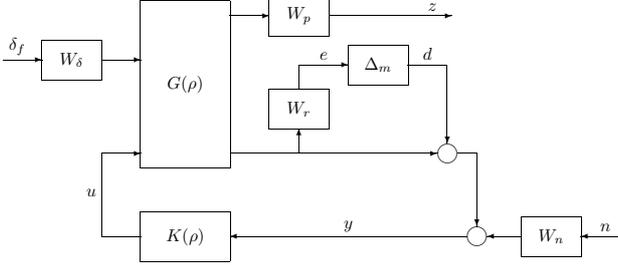
Figure 2: The closed-loop interconnection structure
