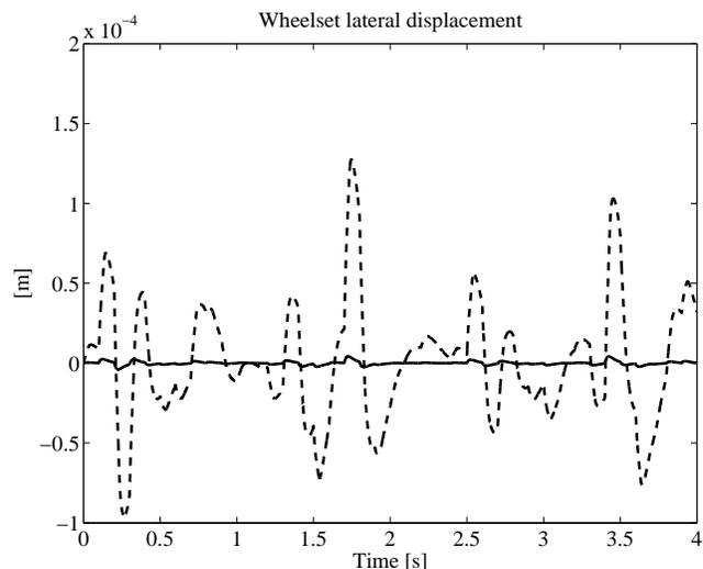
Figure 3: Closed-loop front wheelset lateral displacement (front bogie). Solid line: colocated feedback; dashed line: non-colocated feedback.
