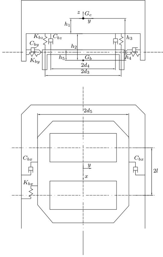
Figure 2: Half a car with bogie.
