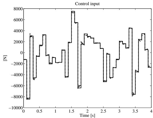
Figure 5: Control input: front wheelset, front bogie. Solid line: collocated feedback; dashed line: noncollocated feedback.
