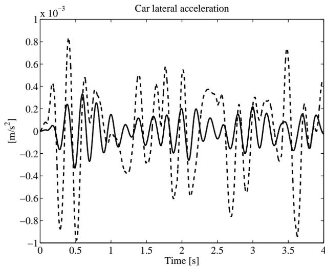
Figure 4: Closed-loop car lateral acceleration. Solid line: collocated feedback; dashed line: noncollocated feedback.
