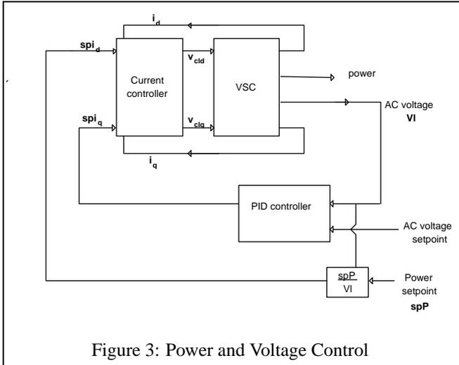
Figure 3: Power and Voltage Control
