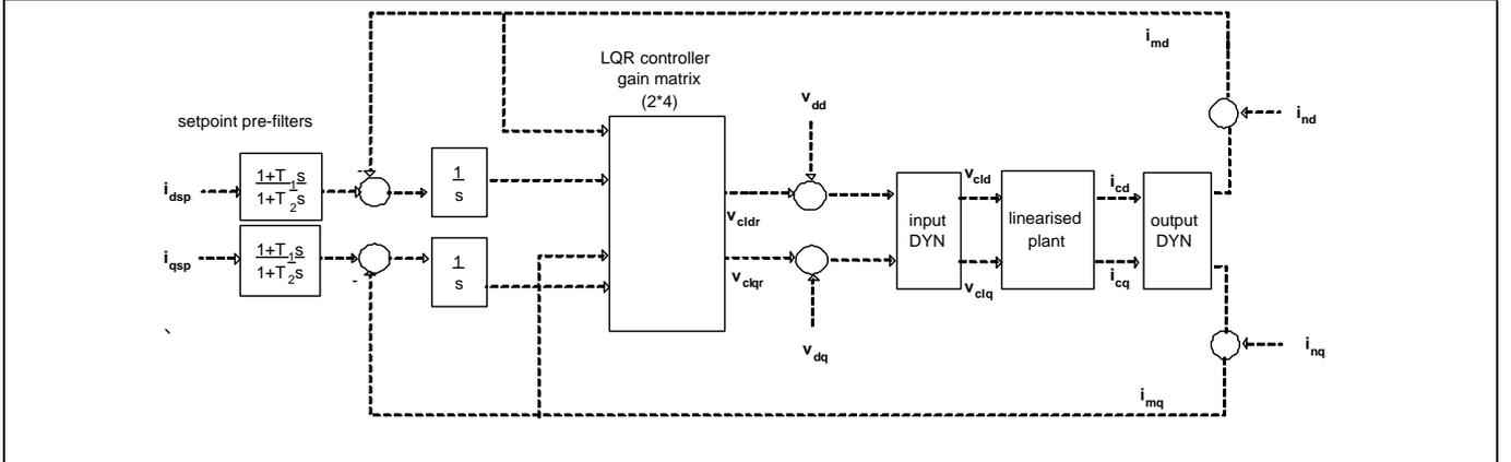
Figure 2: LQR Control structure for VSC
