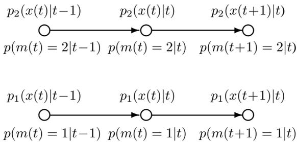
Figure 1: State filtering and model classification with parallel models
