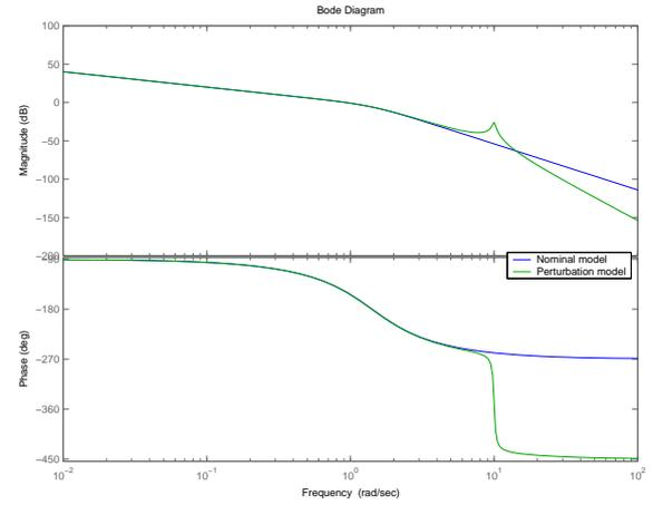
Figure 8: Bode diagrams - nominal and perturbation model
