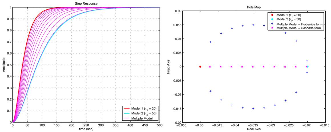
Figure 2: Mixture model step responses and pole map
