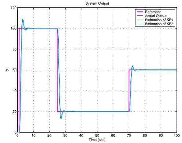
Figure 9: Reference tracking - deterministic simulation
