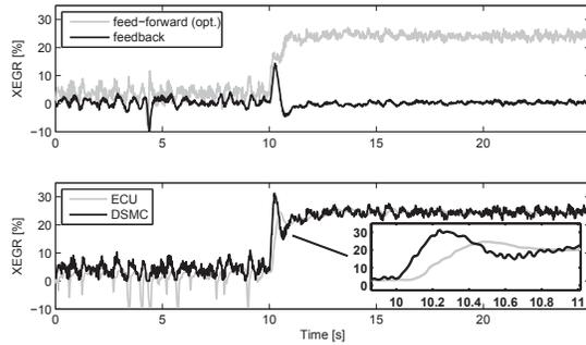
Fig. 9. EGR valve control signal with optimized feed forward part
