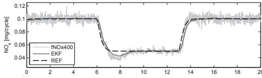
Fig. 6. NO<sub>x</sub> tracking with sliding mode method -  $Wf = 10\text{mg/cycle}$  and  $N = 1700\text{rpm}$
