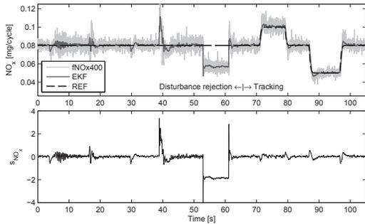
Fig. 5. Disturbance rejection and tracking done by Discrete time Sliding Mode Control (DSMC)
