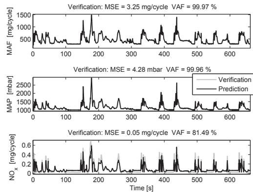
Fig. 4. Outputs for NARX model verification - Part of FTP75
