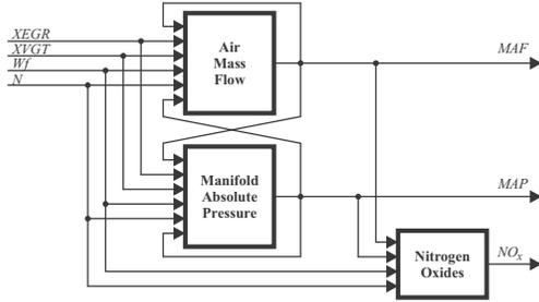
Fig. 1. Air path and  $\text{NO}_x$  model structure
