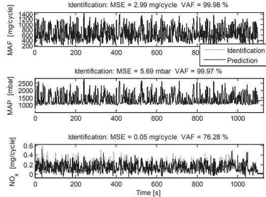
Fig. 2. NARX identification with predicted and measured output signals (MSE - mean square error, VAF - variance accounted for)
