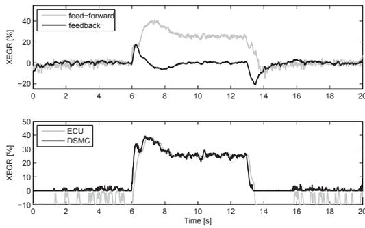
Fig. 7. Manipulated XEGR signal from the sliding mode controller
