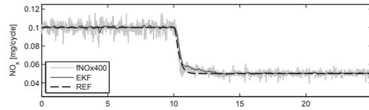
Fig. 8. NO<sub>x</sub> tracking and switching function with sliding mode method and optimized feed forward part -  $Wf = 10\text{mg/cycle}$  and  $N = 1700\text{rpm}$
