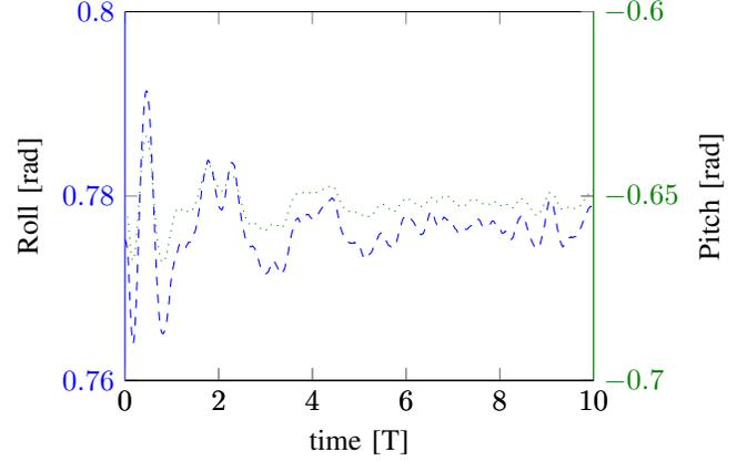
Fig. 9. Time traces of the Cubli's roll( $\gamma$ ) and pitch( $\beta$ ) during a corner balancing experiment. The non zero converging values correspond to the constant bias in attitude measurements.
