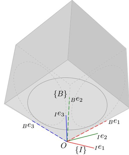
Fig. 5. Cubli balancing on the corner.  ${}^B e_*$  and  ${}^I e_*$  denote the principle axis of the body fixed frame  $\{B\}$  and inertial frame  $\{I\}$ . The pivot point  $O$  is the common origin of coordinate frames  $\{I\}$  and  $\{B\}$ .
