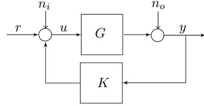
Fig. 7. The block diagram of the system identification procedure: The edge balancing system  $G$  is controlled by a nominal linear feedback controller  $K$  and is excited by the random phase multisine signal  $r$ .  $n_i$  and  $n_o$  denote the Gaussian white noise on the input and output of the system.
